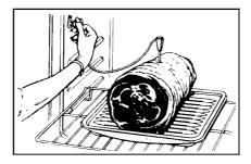
**Step 3:** Plug cable into receptacle on oven wall. The prongs are especially designed to only plug in one way. Be certain to insert plug into receptacle all the way. Close oven door.
